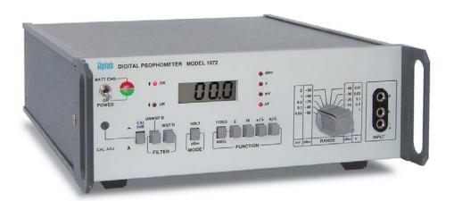
**Aplab Psophometer** is a portable unit designed for the use of testing telecommunication equipment. It has Psophometric filter, which has the frequency response of the weighing network based on the CCITT recommendations and frequency response characteristics for unweighted measurements.
