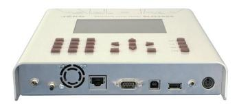
The SLM3505 was designed to provide a single instrument solution for the Electric Utility System Protection Engineer and Relay/Communications Technician responsible for the alignment and maintenance of Power Line Carrier, Audio Tone and FSK Communications Systems. This multifunction instrument replaces all 4 existing Power Line Carrier Instruments in one for a fraction of the cost, all in a compact lightweight package.
